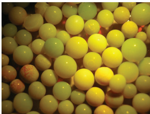
Fig. 5 An example of a SILP containing chlorocuprate(II) ionic liquid impregnated porous 4 mm diameter silica spheres.
